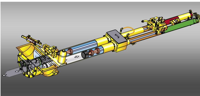
This open loop **Generation 3** all-hydraulic concrete pump sets the standard for fuel-efficiency, reliability and performance. Twin circuit hydraulics combine with the longest stroking pumping cylinders in the industry for a smooth, continuous flow of concrete which also translates to longer boom life. **Big Rock Valve** is designed to pump the harshest mixes and provide the lowest per yard operating costs.
