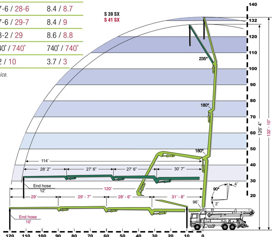
S 39 SX / S 41 SX (Dimensions shown apply to Mack truck mounted units and may vary unit to unit or for other makes and models of trucks.)
