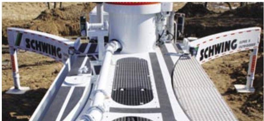
*Super X outriggers are a Schwing exclusive providing maximum stability with the smallest footprint. These telescopic, single-stage outriggers set-up fast and don't extend in front of the cab for maximum horizontal boom reach.*
